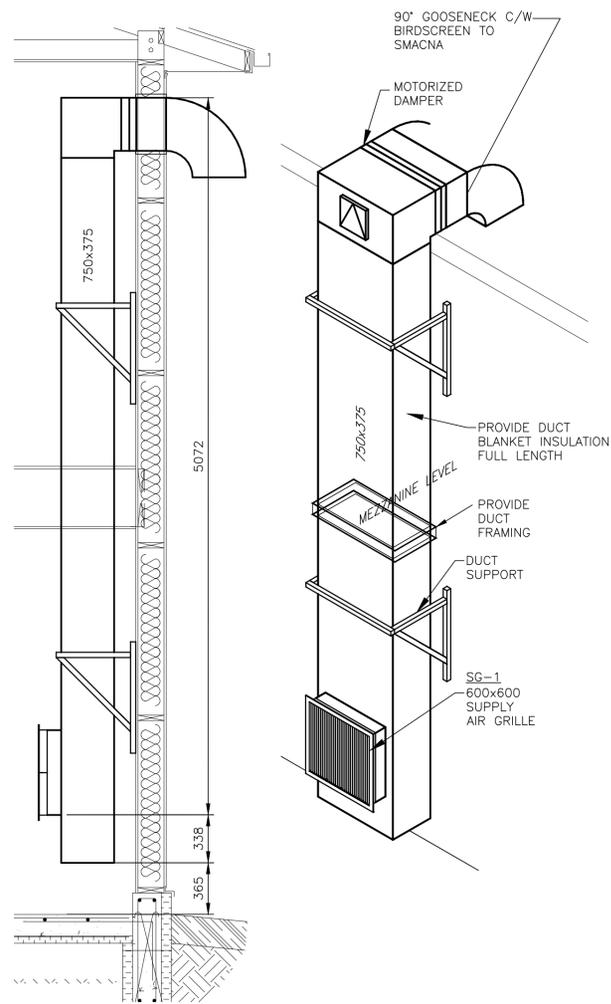
**A** DETAIL - O/A INTAKE DUCT TYP.
