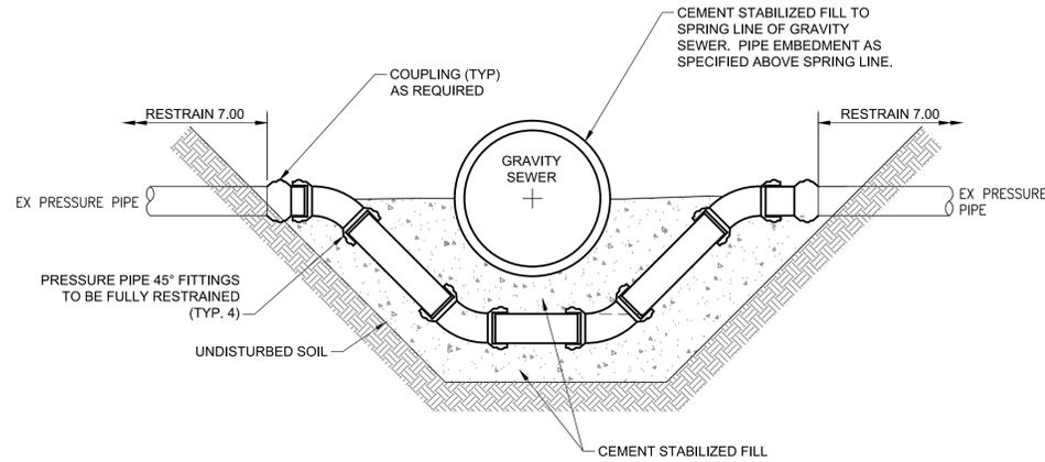
**VERTICAL RE-ALIGNMENT OF PRESSURE PIPE DETAIL**
