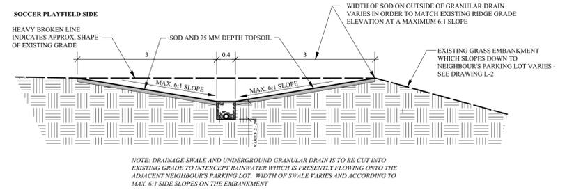
7 FIELD 2 WEST GRANULAR DRAIN SECTION
