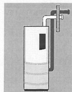
Sealed Direct Vent—sidewall
