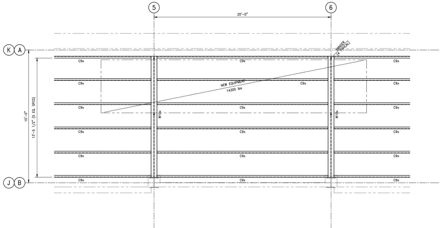
**A** PARTIAL CATWALK FLOOR PLAN - DESIGN FLOOR LIVE LOAD - 25 psf
