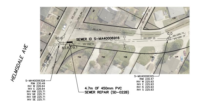
SEWER JUNCTION INFORMATION FROM SEWER VIDEO INSPECTION SEWER ID S-MA40006916 DISTANCE FROM MH ID S-MH40006325 DISTANCE DIAMETER CLOCK 150 37.0 150
