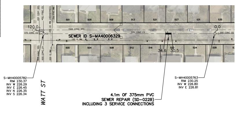
SEWER JUNCTION INFORMATION FROM SEWER VIDEO INSPECTION SEWER ID S-MA40006329 DISTANCE FROM MH ID S-MH40005763 DISTANCE DIAMETER CLOCK 1.2 150 10 2.7 150 11.9 150 11 18.5 100 32.6 150 10 33.2 150 34.5 150 43.7 150 48.6 150 11 \*\*\*\*REVERSAL REQUIRED\*\*\*\*
