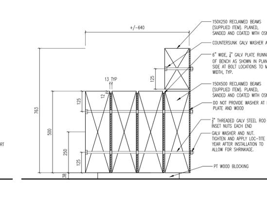
10 INTERIOR WOOD BENCH AT HIGH SEAT - SECTION 1:10 (of 24X36)
