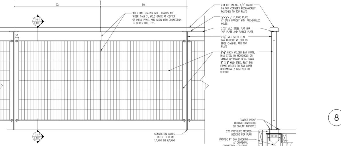
5 GUARDRAIL ELEVATION, TYP. 1:10 (of 24X36)
