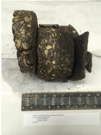
**CORE #CH02 – ASPHALT SECTION**
