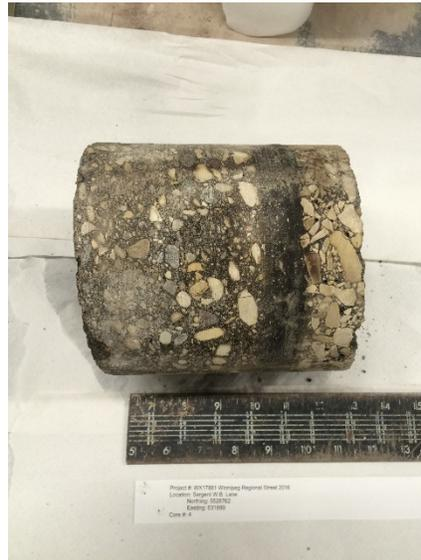
**CORE #CH04 – ASPHALT SECTION**
