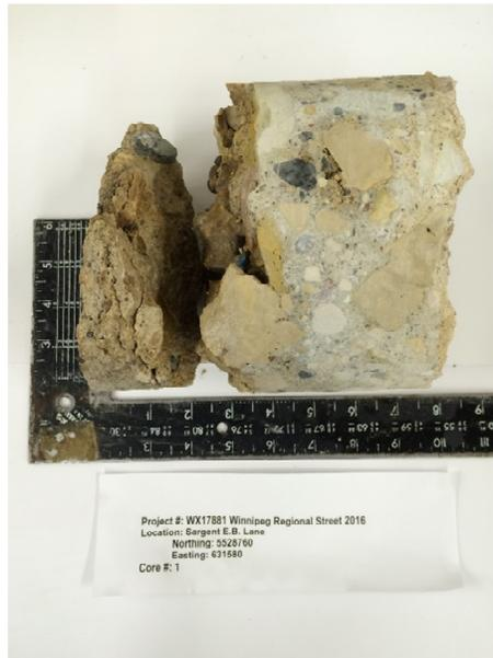
**CORE #CH01 – CONCRETE SECTION**
