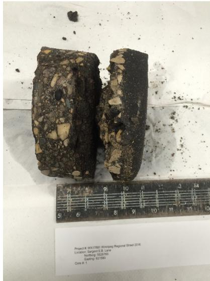
**CORE #CH01 – ASPHALT SECTION**
