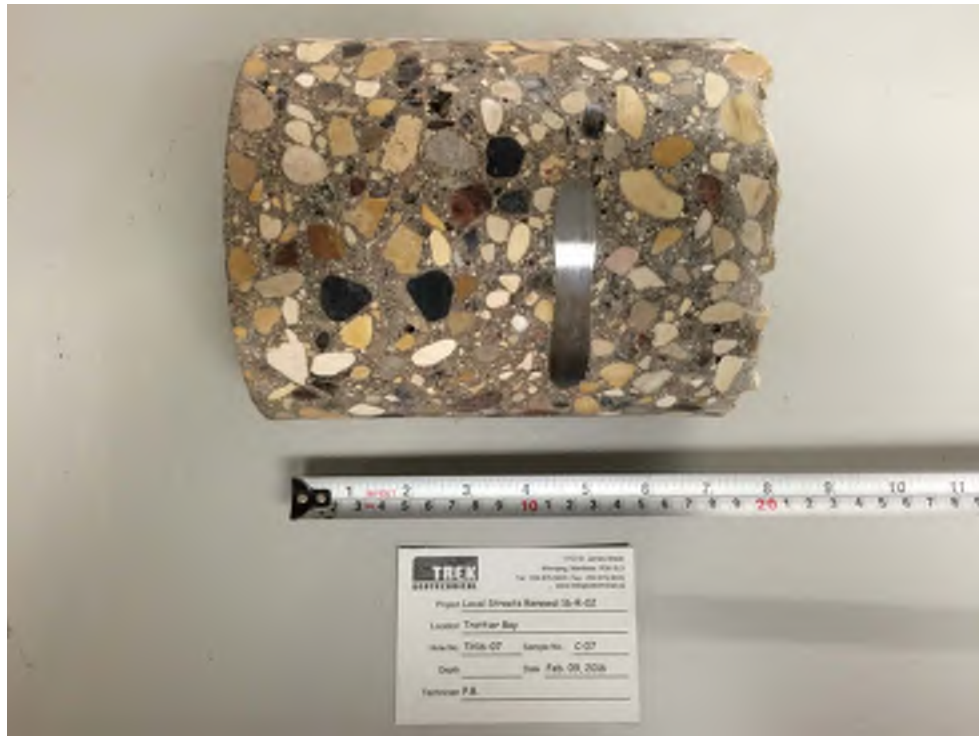
Photo 7: Pavement Core Sample at Test Hole TH16-07
