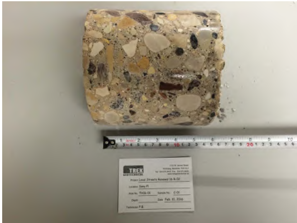
Photo 1: Pavement Core Sample at Test Hole TH16-01
