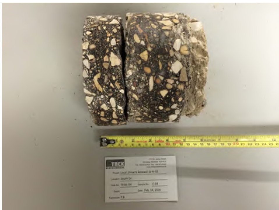
Photo 4: Pavement Core Sample at Test Hole TH16-04
