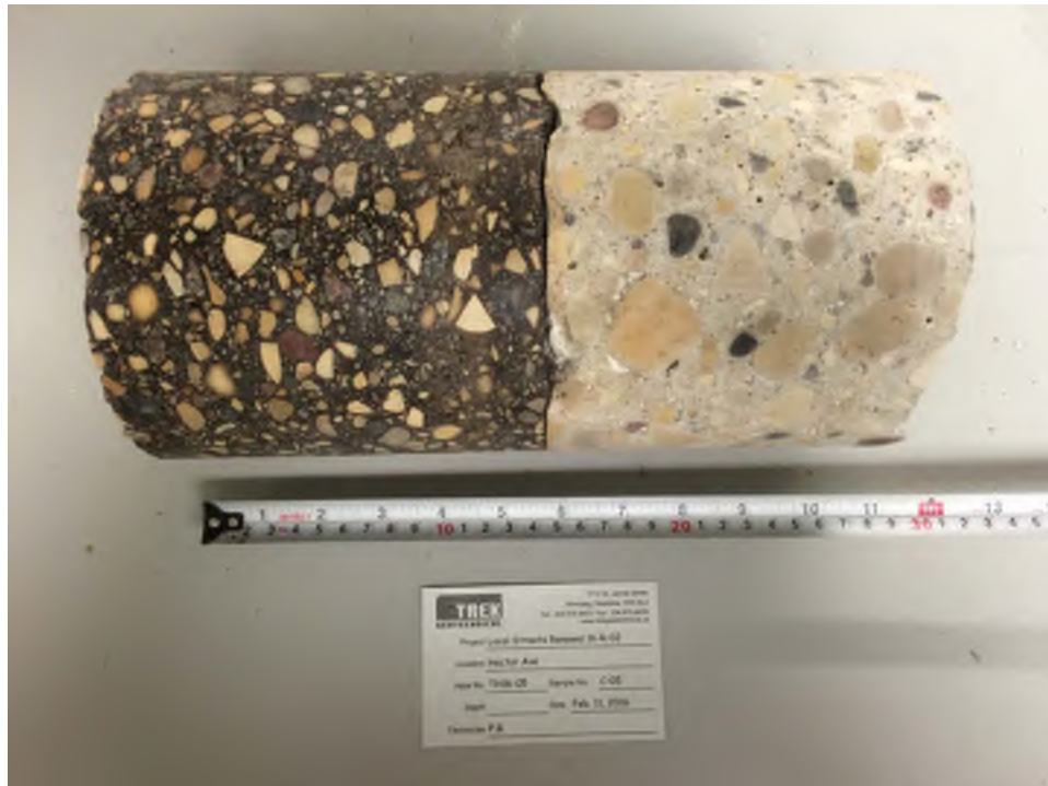
Photo 5: Pavement Core Sample at Test Hole TH16-05
