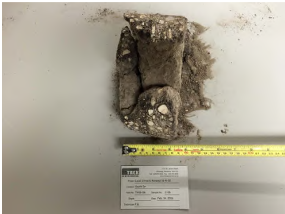
Photo 6: Pavement Core Sample at Test Hole TH16-06
