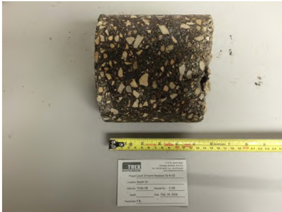
Photo 5: Pavement Core Sample at Test Hole TH16-05
