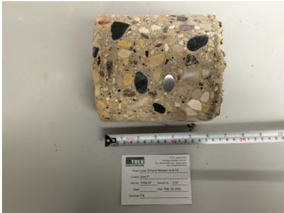
Photo 7: Pavement Core Sample at Test Hole TH16-07
