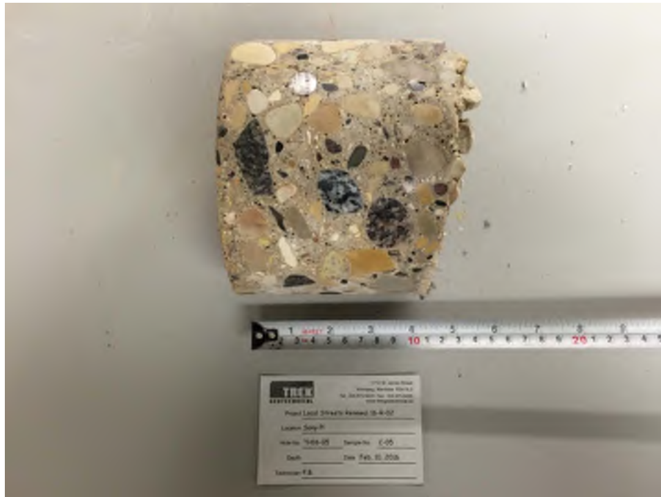
Photo 5: Pavement Core Sample at Test Hole TH16-05
