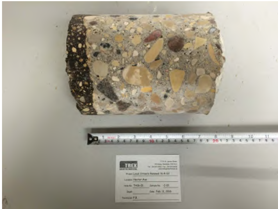
Photo 1: Pavement Core Sample at Test Hole TH16-01
