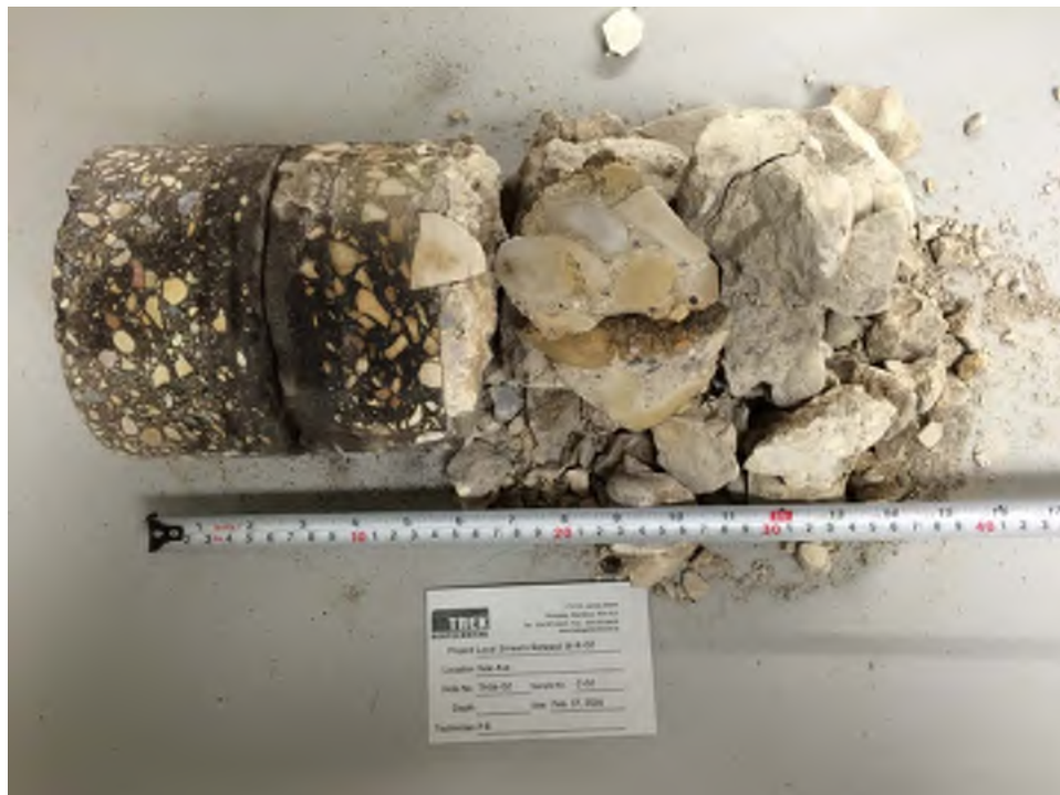
Photo 2: Pavement Core Sample at Test Hole TH16-02
