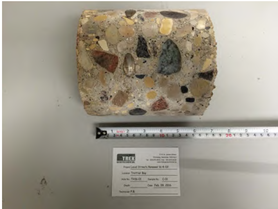
Photo 1: Pavement Core Sample at Test Hole TH16-01
