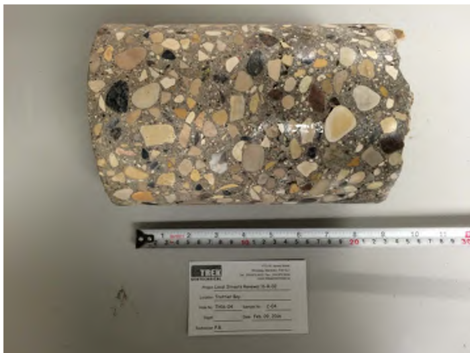
Photo 4: Pavement Core Sample at Test Hole TH16-04
