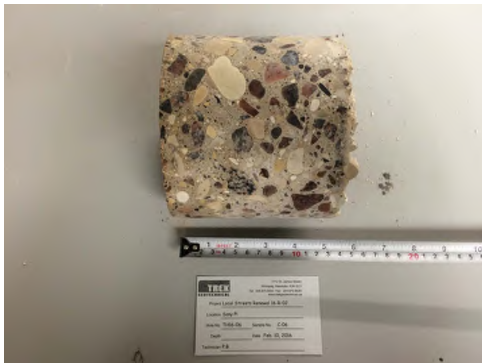
Photo 6: Pavement Core Sample at Test Hole TH16-06
