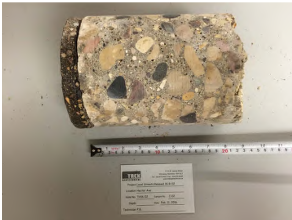
Photo 2: Pavement Core Sample at Test Hole TH16-02
