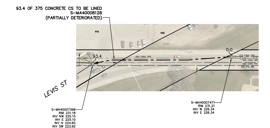
SEWER JUNCTION INFORMATION FROM SEWER VIDEO INSPECTION SEWER ID S-MA40008128 DISTANCE FROM MH ID S-MH40007471 DISTANCE DIAMETER CLOCK 77.4 100
