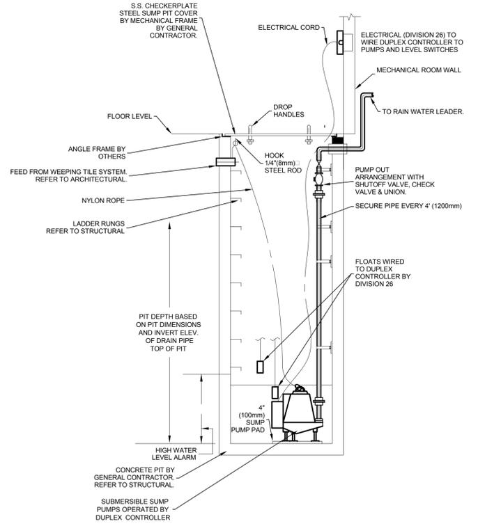
6 SUMP PUMP DETAIL - STRUCTURAL PIT
