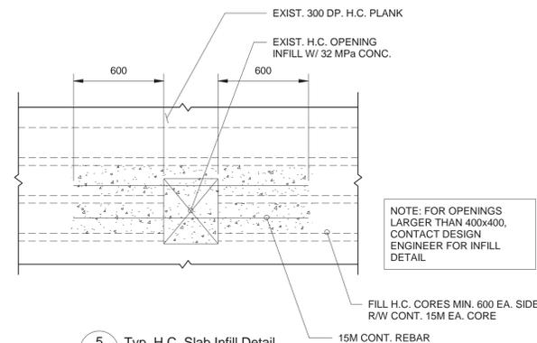
5 Typ. H.C. Slab Infill Detail
