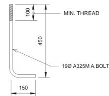
4 Typ. Anchor Bolt Detail
