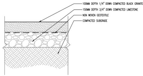
**1 COMPACTED AGGREGATE SURFACING, TYP.**
