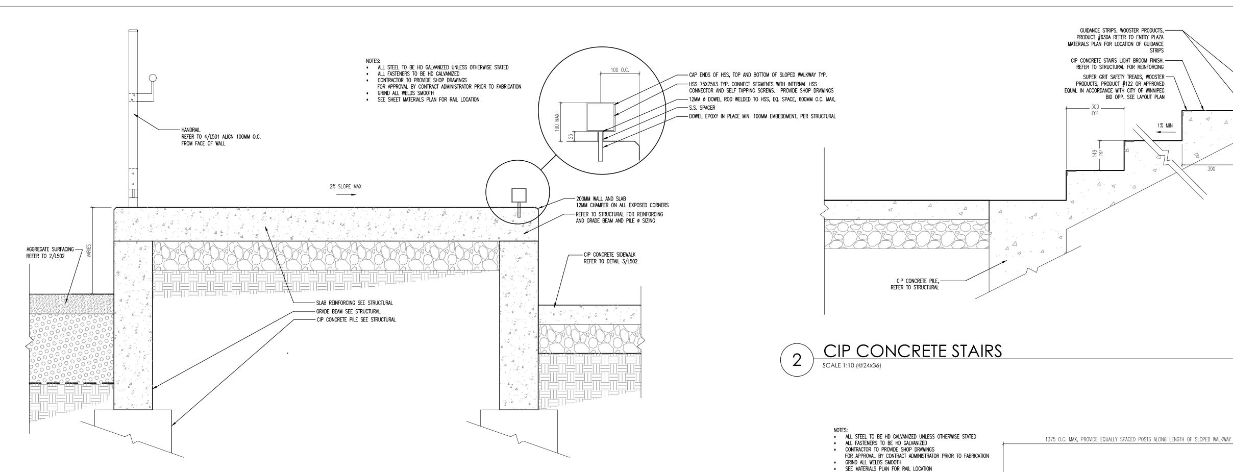
CIP CONCRETE SLOPED WALK-WAY W/ BULL-RAIL & RAILING
