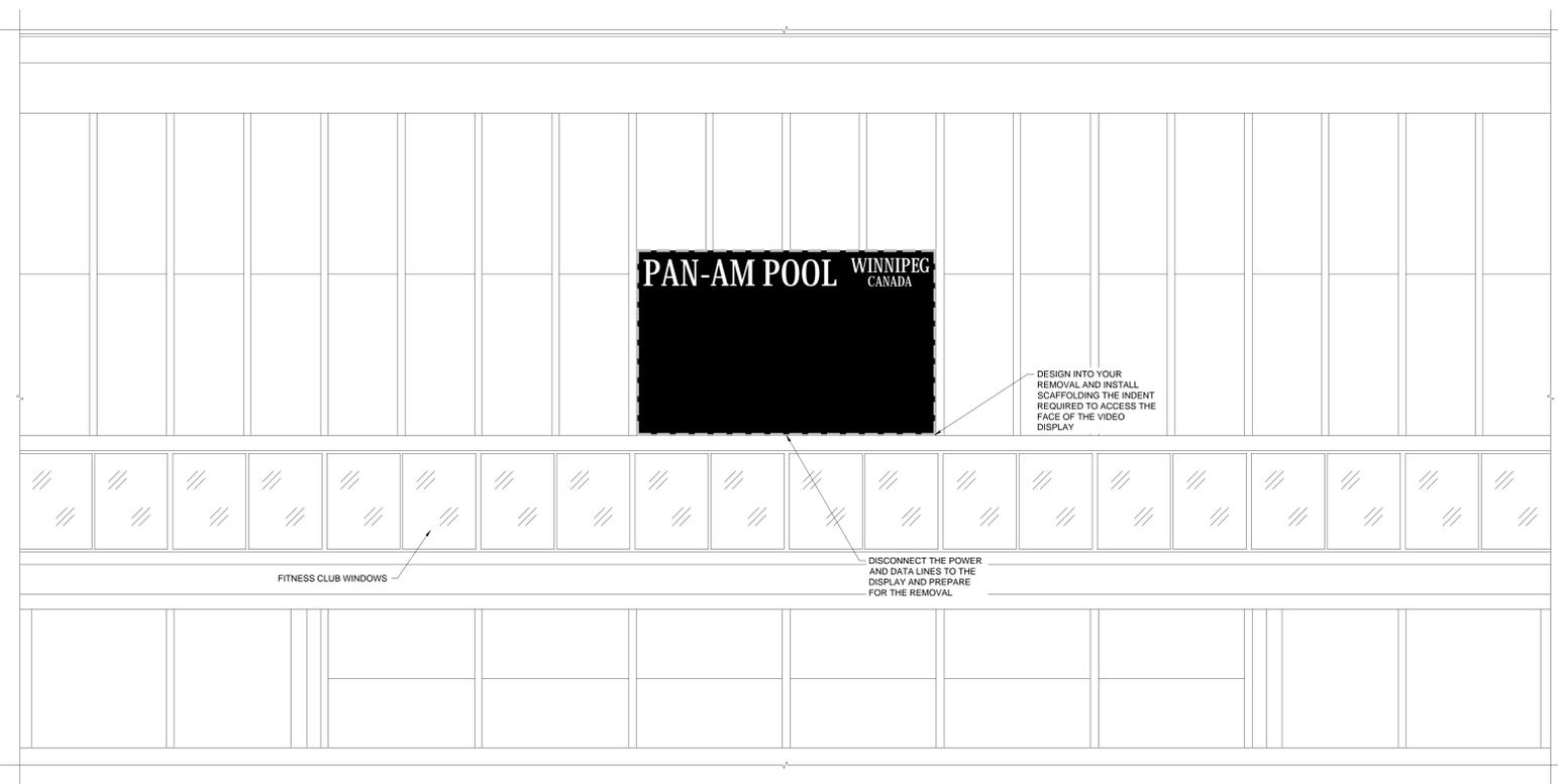
DISPLAY - REMOVAL OF THE EXISTING BOARD - ELEVATION 2 NOT TO SCALE AQ101
