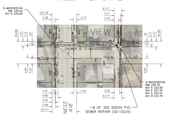
SEWER JUNCTION INFORMATION FROM SEWER VIDEO INSPECTION SEWER ID S-MA20000195 DISTANCE FROM MH ID S-MH20000144 DISTANCE DIAMETER CLOCK 200 10
