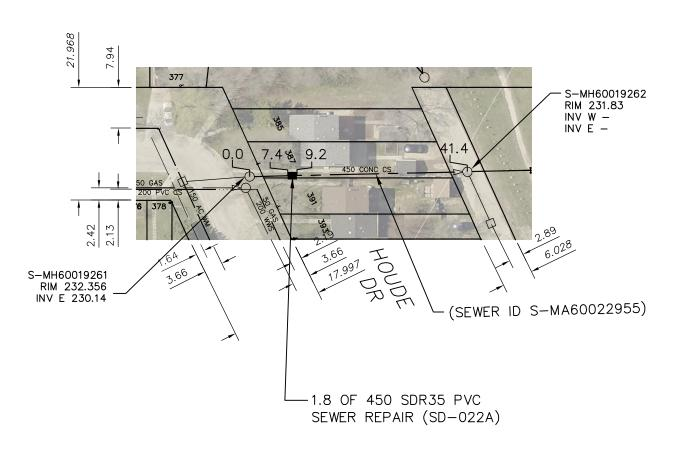
SEWER JUNCTION INFORMATION FROM SEWER VIDEO INSPECTION SEWER ID S-MA60022955 DISTANCE FROM MH ID S-MH60019261 DISTANCE DIAMETER CLOCK \*\*\* NO SERVICE JUNCTIONS \*\*\*\*
