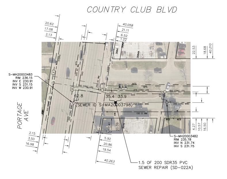
SEWER JUNCTION INFORMATION FROM SEWER VIDEO INSPECTION SEWER ID S-MA20003798 DISTANCE FROM MH ID S-MH20003482 DISTANCE DIAMETER 150 16.5
