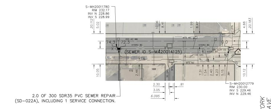
SEWER JUNCTION INFORMATION FROM SEWER VIDEO INSPECTION SEWER ID S-MA20014125 DISTANCE FROM MH ID S-MH20012779 DISTANCE DIAMETER CLOCK 10 6.3 9.3 150 20.4 150 150 21.1 36.4 150 37.8 38.5 40.2 150 40.7 150 42.4 150 10 49.5 150 9 50.1 150 66.8 150 67.5 150 72.4 150
