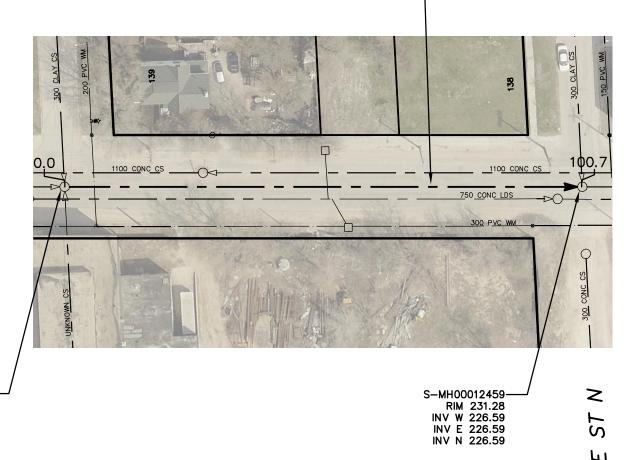
SEWER JUNCTION INFORMATION FROM SEWER VIDEO INSPECTION SEWER ID S-MA00013960 DISTANCE FROM MH ID S-MH00012451 DISTANCE DIAMETER 5.9 150 10 16.6 150 16.8 150 24.6 150 150 24.8 32.2 150 32.4 150 32.6 150 \*\*\*\*REVERSAL REQUIRED\*\*\*\*
