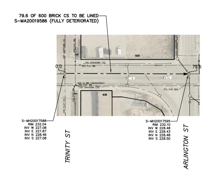
SEWER JUNCTION INFORMATION FROM SEWER VIDEO INSPECTION SEWER ID S-MA20019586 DISTANCE FROM MH ID S-MH20017588 DISTANCE DIAMETER CLOCK 150 8.8 12.0 150 150 16.0 20.0 150 10 24.4 200 35.5 150 36.8 150 40.2 200 41.1 200 10 44.1 150 10 50.6 150 50.7 150 10 52.7 200 150 65.8 10 150 150 65.9 69.4 70.9 150
