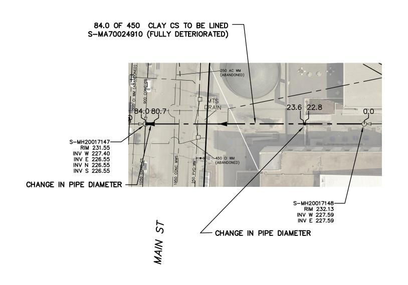
SEWER JUNCTION INFORMATION FROM SEWER VIDEO INSPECTION SEWER ID S-MA70024910 DISTANCE FROM MH ID S-MH20017148 DISTANCE DIAMETER 4.6 150 5.1 150 10 5.8 150 150 10 6.4 20.7 150 21.5 150 10 150 25.1 30.4 150 10 31.5 150 10 150 46.8 48.5 150 12 49.4 150 53.8 150 57.0 150 59.7 150 60.7 150 11 61.3 150 62.4 150 72.3 150 73.4 150 10 74.1 150 11 150 11
