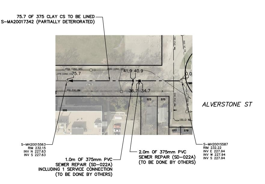
SEWER JUNCTION INFORMATION FROM SEWER VIDEO INSPECTION SEWER ID S-MA20017342 DISTANCE FROM MH ID S-MH20015587 DISTANCE DIAMETER 9.3 150 10 10.1 150 10 22.7 27.6 150 11 150 38.3 150 10 41.4 150 10 42.1 150 44.9 150 10 60.3 150 10 150 67.7 68.4 150 10 72.2 150 72.6 200 11
