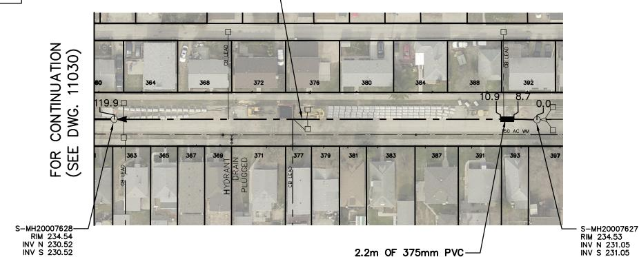
SEWER JUNCTION INFORMATION FROM SEWER VIDEO INSPECTION SEWER ID S-MA20008297 DISTANCE FROM MH ID S-MH20007628 DISTANCE DIAMETER CLOCK 12 1.6 150 1.9 150 10 2.4 150 7.8 150 10 18.7 150 22.6 150 24.8 150 11 25.6 150 26.3 150 10 32.5 150 10 32.7 150 36.0 150 10 36.6 150 2 38.0 150 10 40.4 150 47.5 150 52.0 150 12 54.5 150 10 55.3 150 56.1 150 10 63.3 150 150 68.0 10 70.4 150 10 71.1 150 85.3 150 10 86.0 150 2 100.9 150 10 101.8 150 150 109.5 109.7 150 \*\*\*\*REVERSAL REQUIRED\*\*\*\*
