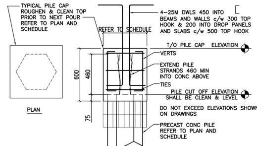
PROVIDE SINGLE CAP DETAIL FOR PILES EXCEEDING PLACEMENT CRITERIA
