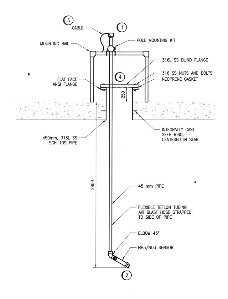
A COVERED TANK ORP SENSOR INSTALLATION NTS
