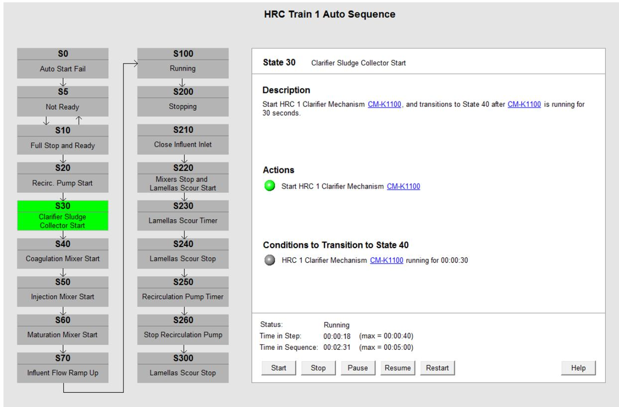
**Figure 2-5: Sample Process Detail Display for a Sequencer**
