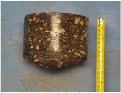
Core sample from Testhole TH4
