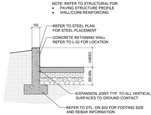
**4** CONCRETE CURB / RETAINING WALL
