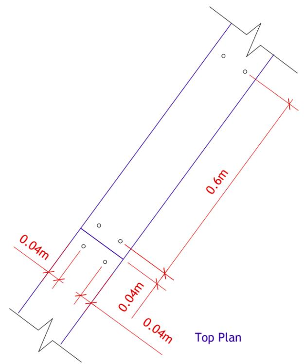
Trex Cap to be predrilled and screwed to Base course using screws. Screws shall be Stainless Steel or Ceramic Coated and approved for use with ACQ treated wood. Screws to extend into timber base a minimum of 5 cm and be countersunk into Trex. Two screws are to be placed at each end and every 60 cm along length. Straight sections of Trex are to be butt jointed.
