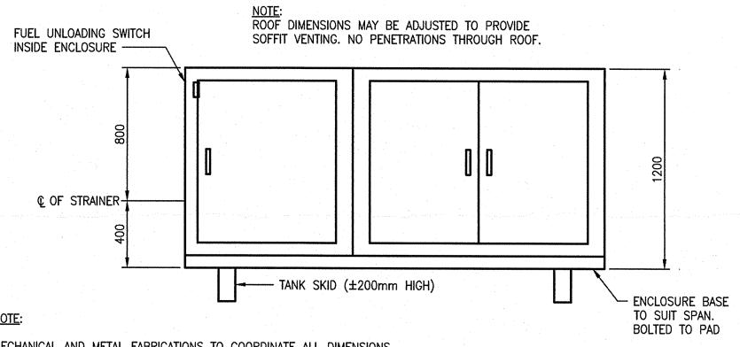
MECHANICAL AND METAL FABRICATIONS TO COORDINATE ALL DIMENSIONS AND DOOR LOCATIONS. SUBMIT SHOP DRAWINGS OF FINAL LAYOUTS FOR ALL ENCLOSURES. REFER SECTION 05 50 00.
