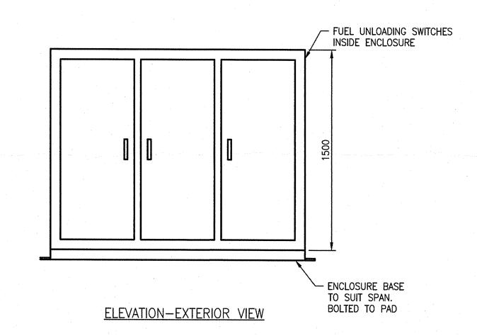
UNLOADING CABINET SERVING COMBINED 8,580L FUEL STORAGE TANK M0007 / SCALE 1:20
