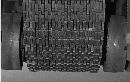
Figure 4 – Saw Blade Cutting Head
