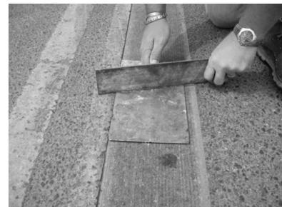
Put straight edge across groove over the top of depth plate
