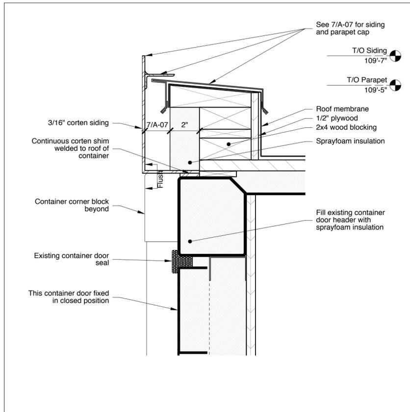
6 Section Detail of Fixed Container Door Header
