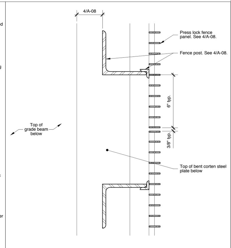
4 Typical Plan Detail of Abutting Fence Panels
