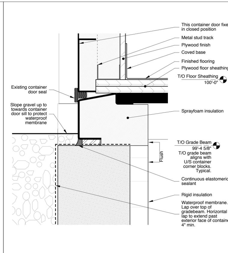
5 Section Detail of Fixed Container Door Sill
