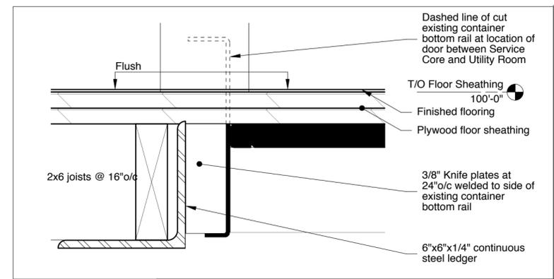
7 Section Detail of Mechanical Core Floor Connection to Containers
