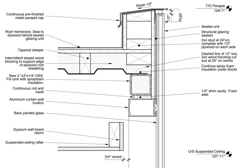
6 Parapet Section Detail at Re-built Container End
