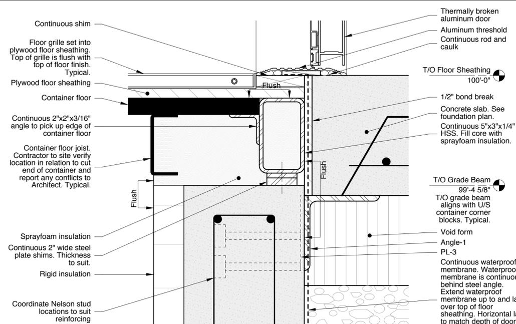
4 Section Detail of Entry Door Sill at Re-built Container End
