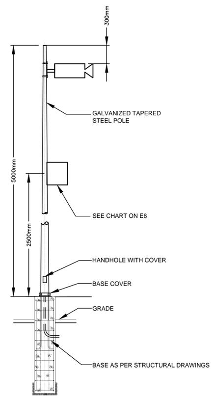
**TYPICAL SECURITY CAMERA POLE MOUNTING DETAIL**
