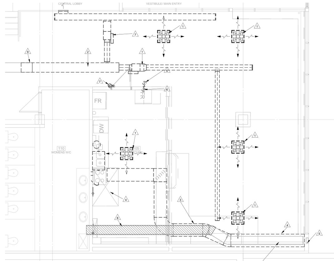
1 MH2.1 MAIN FLOOR HVAC DEMOLITION PARTIAL PLAN - ZONE 1
