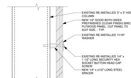
10 PLYWOOD PANEL STANDOFF ASSEMBLY SECTION DETAIL
