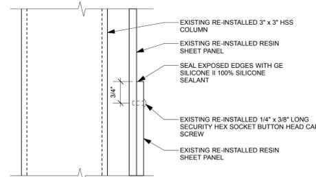
8 TYPICAL RESIN SHEET PANEL CONNECTION DETAIL
