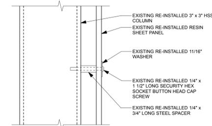
9 RESIN PANEL STANDOFF ASSEMBLY SECTION DETAIL
