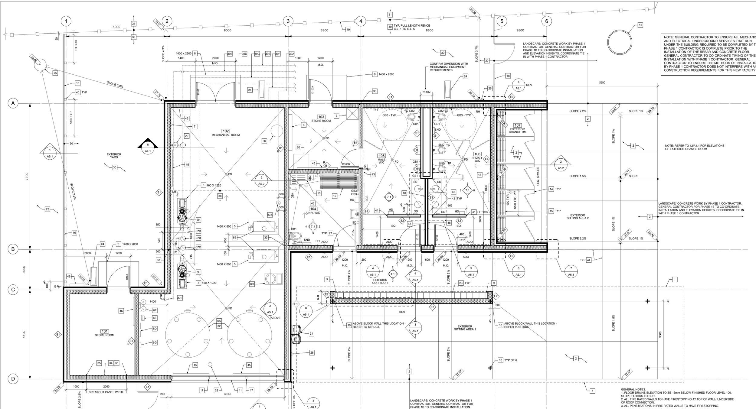
NOTE: GENERAL CONTRACTOR TO ENSURE ALL MECHANICAL AND ELECTRICAL UNDERGROUND SERVICES THAT RUN UNDER THE BUILDING REQUIRED TO BE COMPLETED BY THE PHASE 1 CONTRACTOR IS COMPLETE PRIOR TO THE INSTALLATION OF THE REBAR AND CONCRETE FLOOR. GENERAL CONTRACTOR TO CO-ORDINATE TIMING OF THE INSTALLATION WITH PHASE 1 CONTRACTOR. GENERAL CONTRACTOR TO ENSURE THE METHODS OF INSTALLATION BY PHASE 1 CONTRACTOR DOES NOT INTERFERE WITH ANY CONSTRUCTION REQUIREMENTS FOR THIS NEW FACILITY
