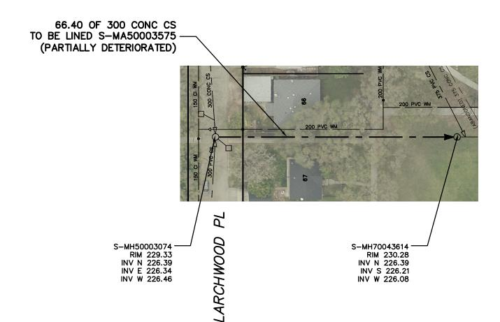
SEWER JUNCTION INFORMATION FROM SEWER VIDEO INSPECTION SEWER ID S-MA50003575 DISTANCE FROM MH ID S-MH50003074 DISTANCE DIAMETER
