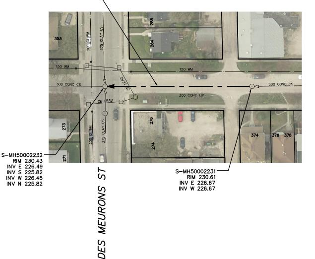
SEWER JUNCTION INFORMATION FROM SEWER VIDEO INSPECTION SEWER ID S-MA50002634 DISTANCE FROM MH ID S-MH50002231 DISTANCE DIAMETER 51.3
