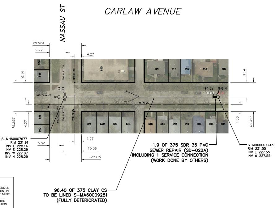
SEWER JUNCTION INFORMATION FROM SEWER VIDEO INSPECTION SEWER ID S-MA60009281 DISTANCE FROM MH ID S-MH60007677 DISTANCE DIAMETER CLOCK 18.7 150 30.5 150 10 43.0 150 45.4 150 10 45.9 150 10 47.4 150 10 57.4 150 63.7 150 10 71.3 150 11 71.9 150 77.6 150 10 86.9 150 94.3 150 10 95.1 150
