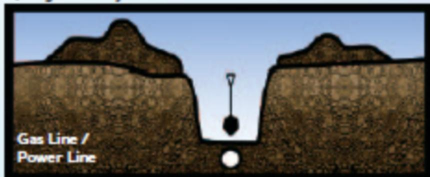
Dig a hole with a shovel directly above the line location until the line is exposed. Take care not to damage the line or coating. Mechanical excavation equipment **MUST NOT** be used to widen or deepen the hole before exposing the line.
