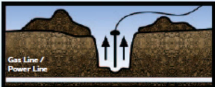
Only oscillating head type nozzles are to be used for the water wand. When excavating within 1 metre horizontally of a marked line the maximum settings of 38°C water temperature and 10,340 Kpa (1,500 psi) must not be exceeded. The end of the vacuum tube shall be neoprene or equivalent. Expose the buried line by using a **SWEEPING MOTION ONLY**, perpendicular to the locate markings, until the line is sighted. After sighting, the line shall not be contacted by spray or vacuum.
