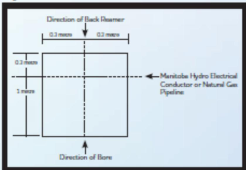
Figure 2: Observation Hole - Profile View
