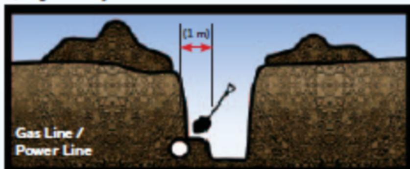
Dig a trench or bell hole 1 metre from the line location, parallel to the line, then hand dig laterally to expose the line.
