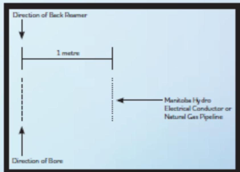
**Figure 5: Drilling Parallel to Manitoba Hydro Conductors and Natural Gas Pipelines - Profile View**
