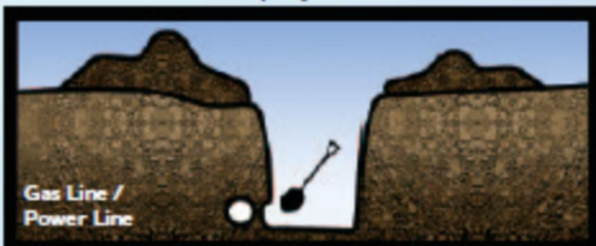
For lines on customer property bringing gas from the main gas pipe to a customer's meter, dig a hole beside the line with a shovel and chip away at the side of the hole to expose the pipe.
