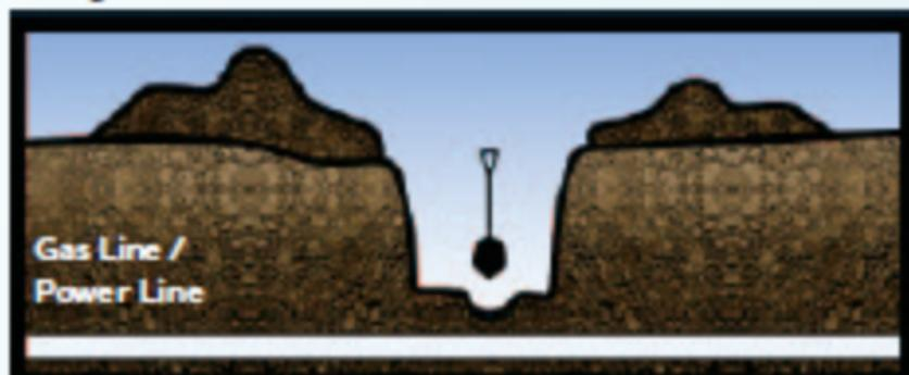
Dig a trench by hand across the full width of the excavation (perpendicular to or "across" the pipe). If the line is not uncovered, mechanically excavate to one half the depth of the trench. Repeat this process until the line is exposed.
