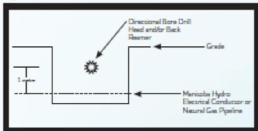
Drilling **above** a Manitoba Hydro electrical conductor or natural gas pipeline.
