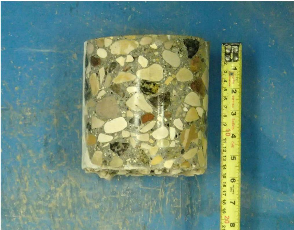
Core sample from Testhole TH2
