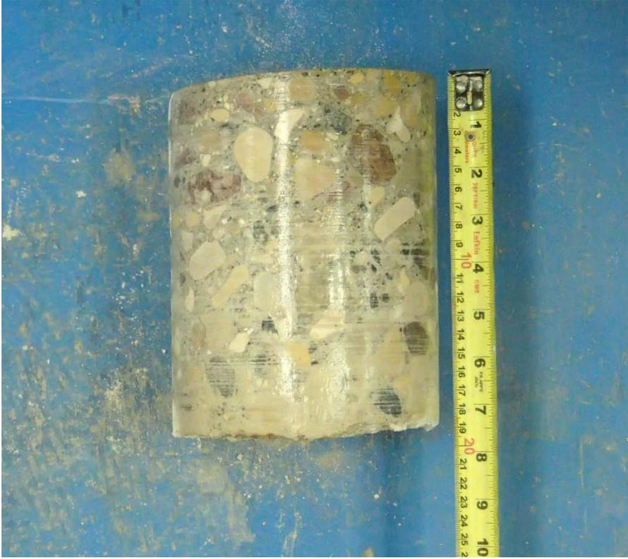
Core sample from Testhole TH2
