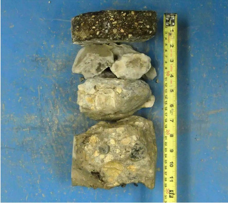
Core sample from Testhole TH1
