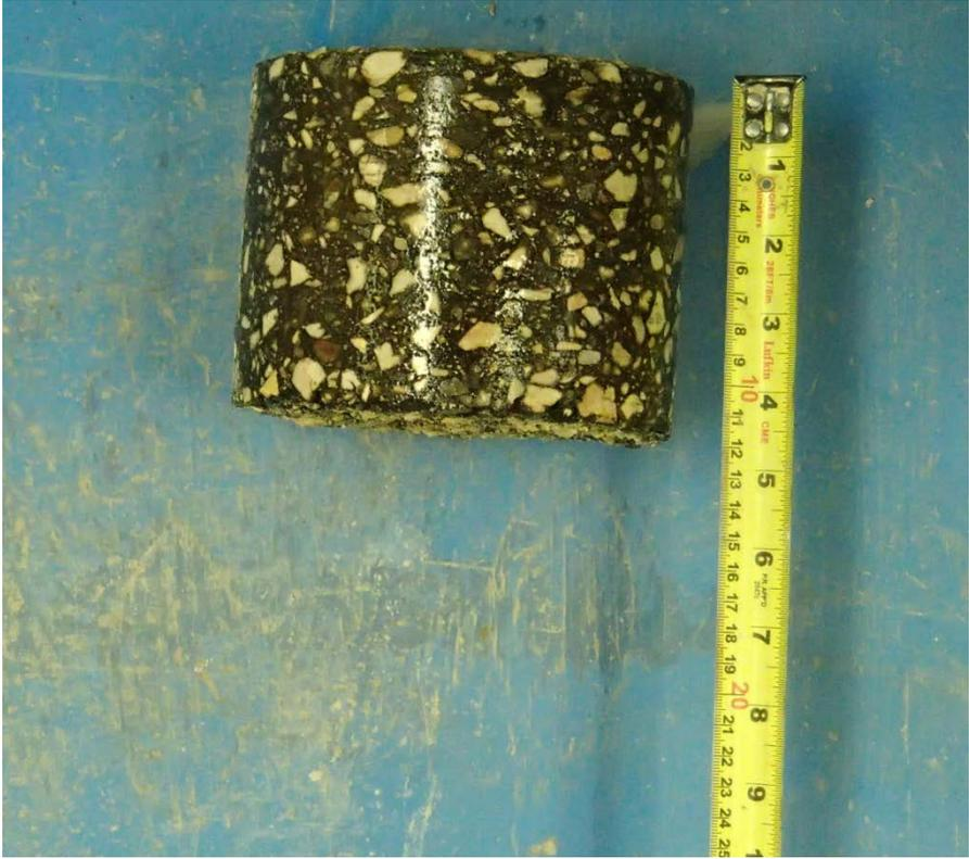
Core sample from Testhole TH3
