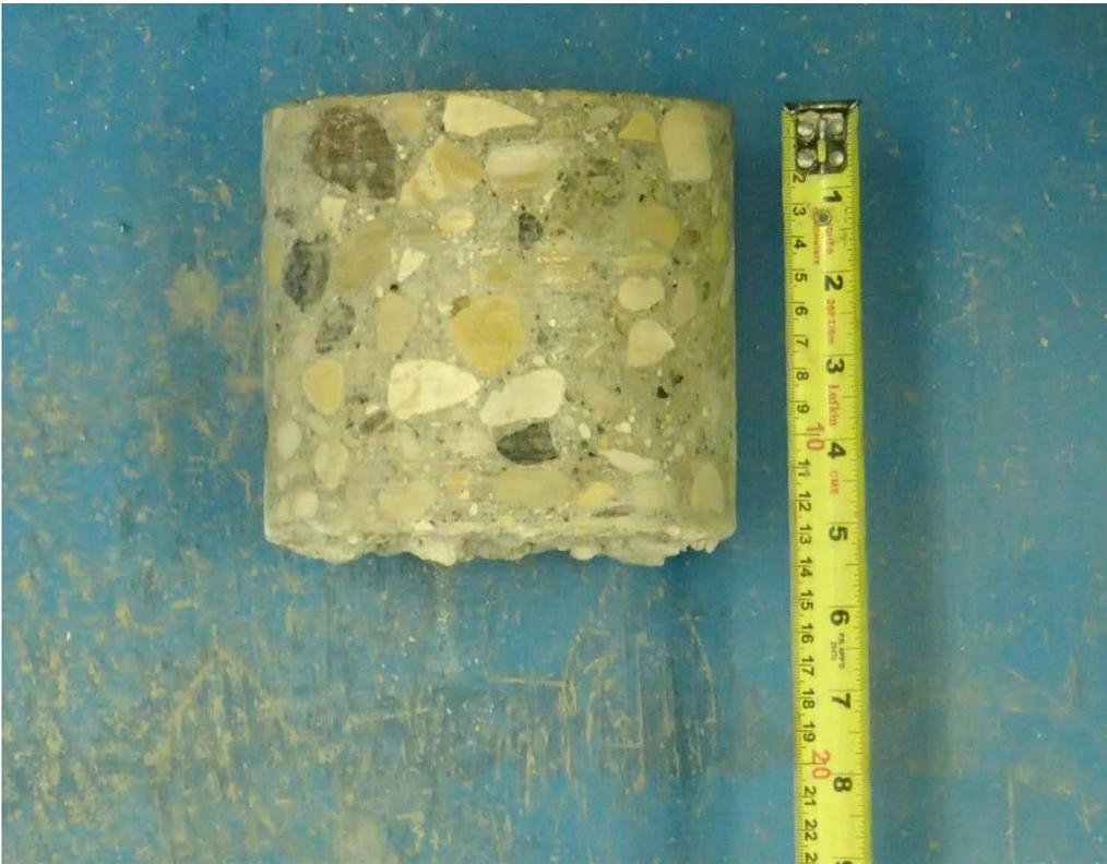
Core sample from Testhole TH2
