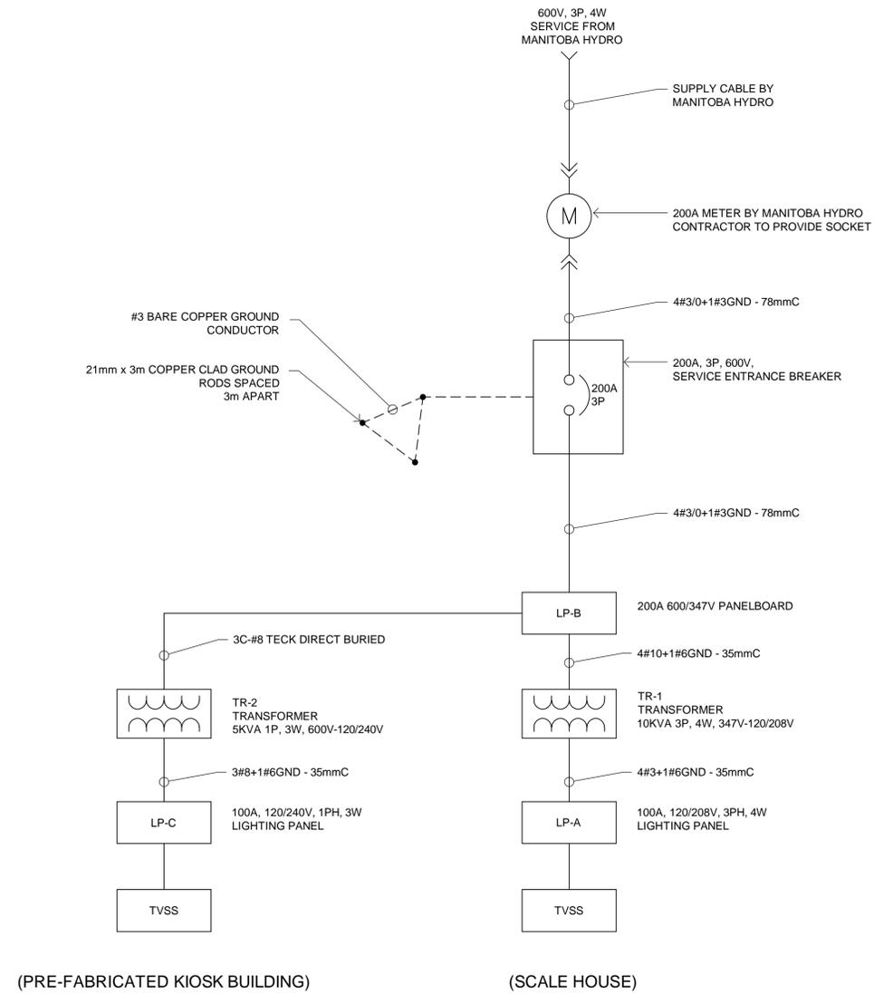
SCALE HOUSE / PRE-FABRICATED KIOSK BUILDING - ONE LINE DIAGRAM
