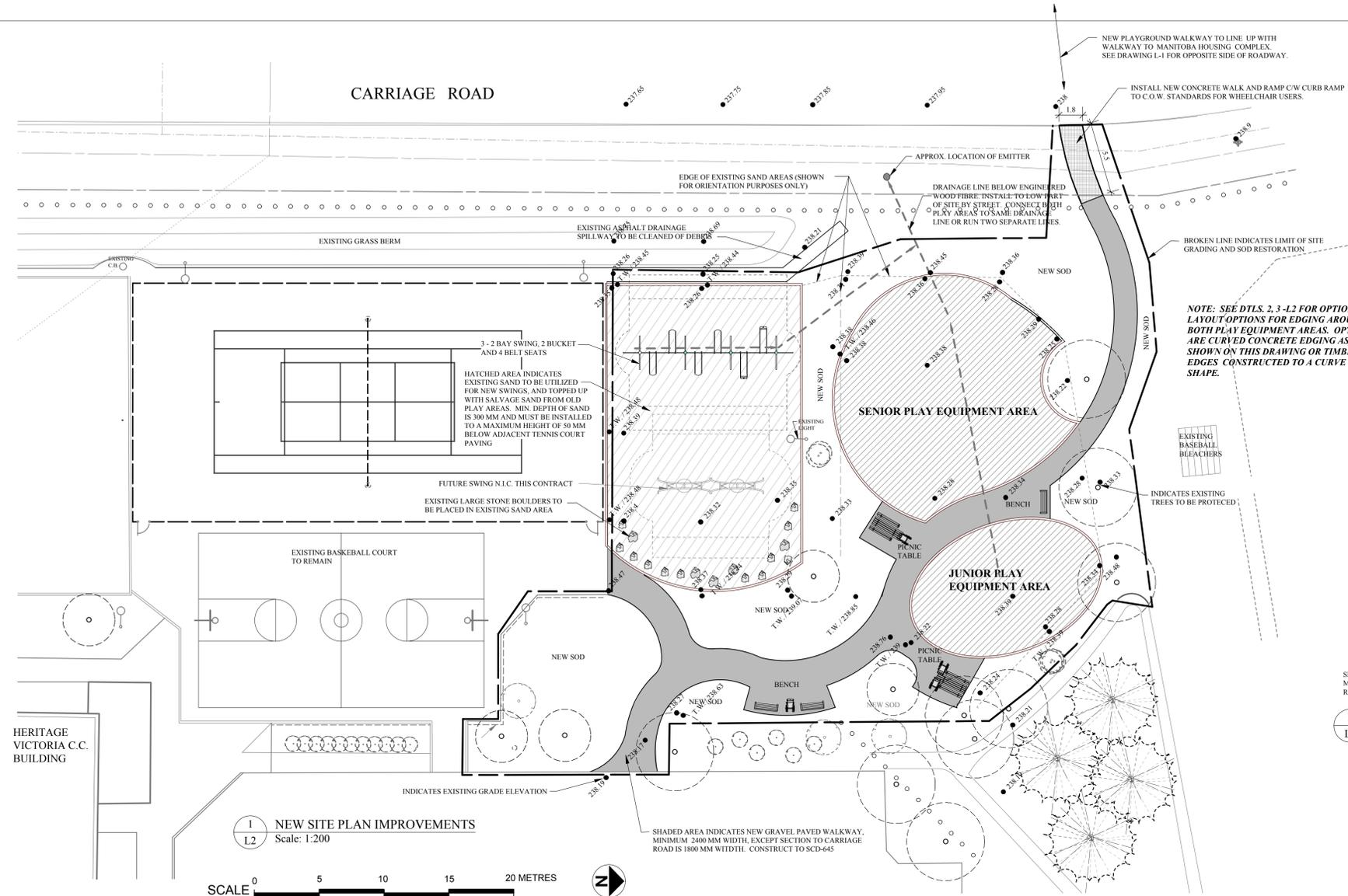
NOTE: SEE DTLS. 2.3-L2 FOR OPTIONAL LAYOUT OPTIONS FOR EDGING AROUND BOTH PLAY EQUIPMENT AREAS. OPTIONS ARE CURVED CONCRETE EDGING AS SHOWN ON THIS DRAWING OR TIMBER EDGES CONSTRUCTED TO A CURVE SHAPE.
