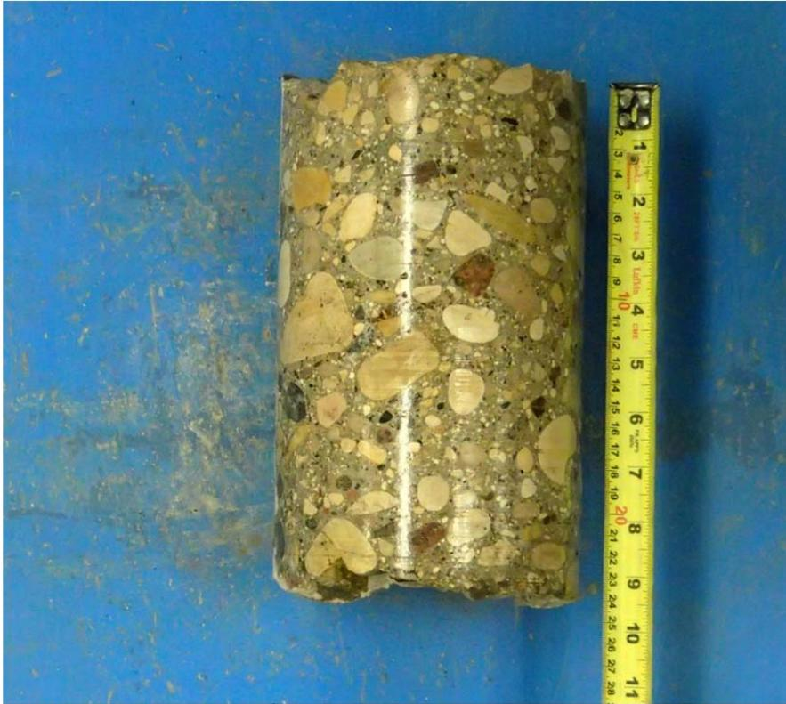
Core sample from Testhole TH1
