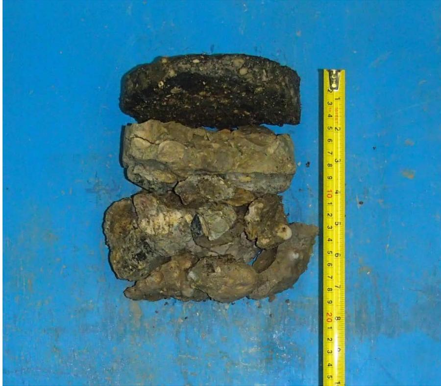
Core sample from Testhole TH1
