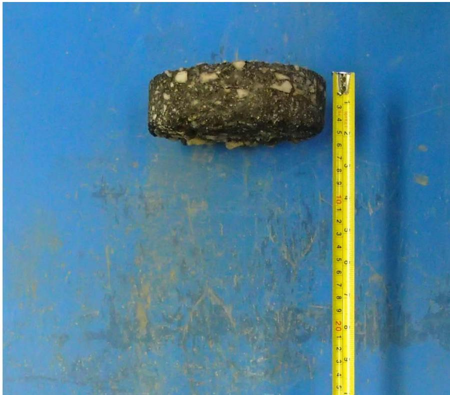
Core sample from Testhole TH2
