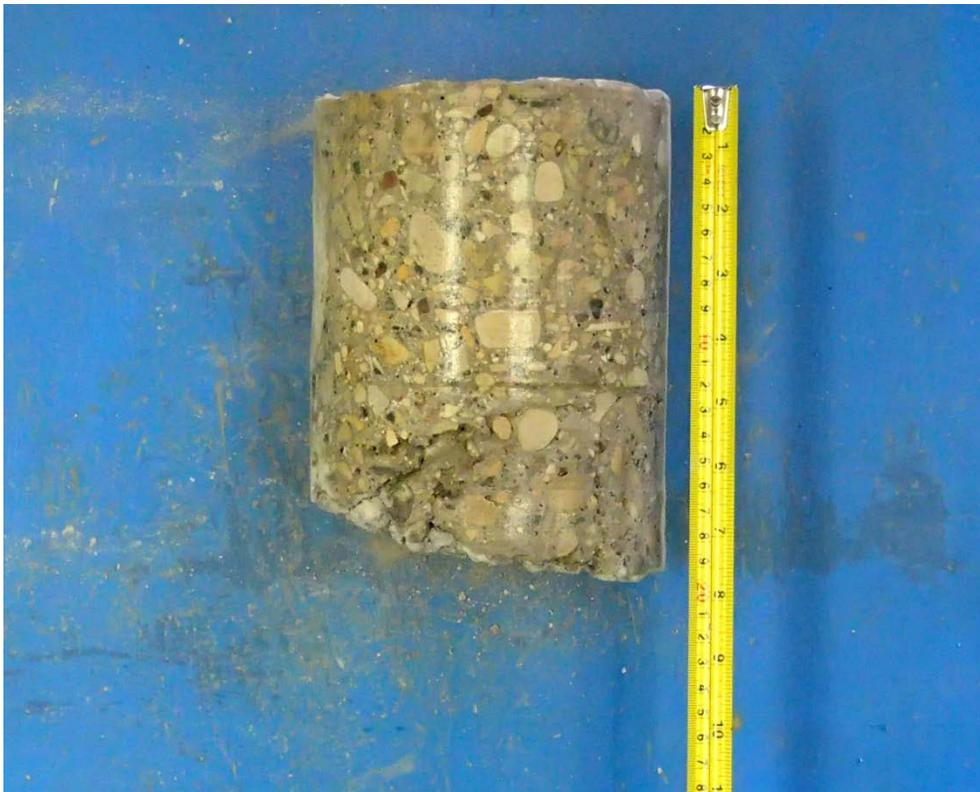
Core sample from Testhole TH8
