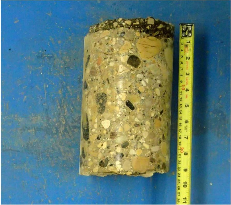
Core sample from Testhole TH7
