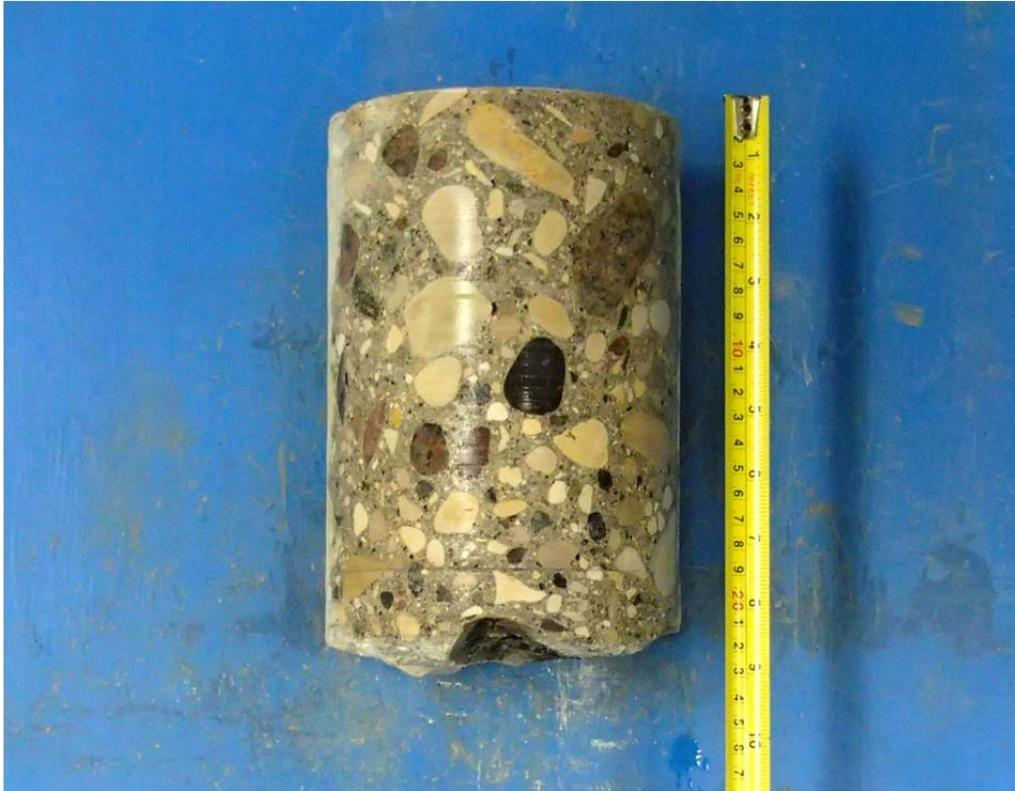
Core sample from Testhole TH3
