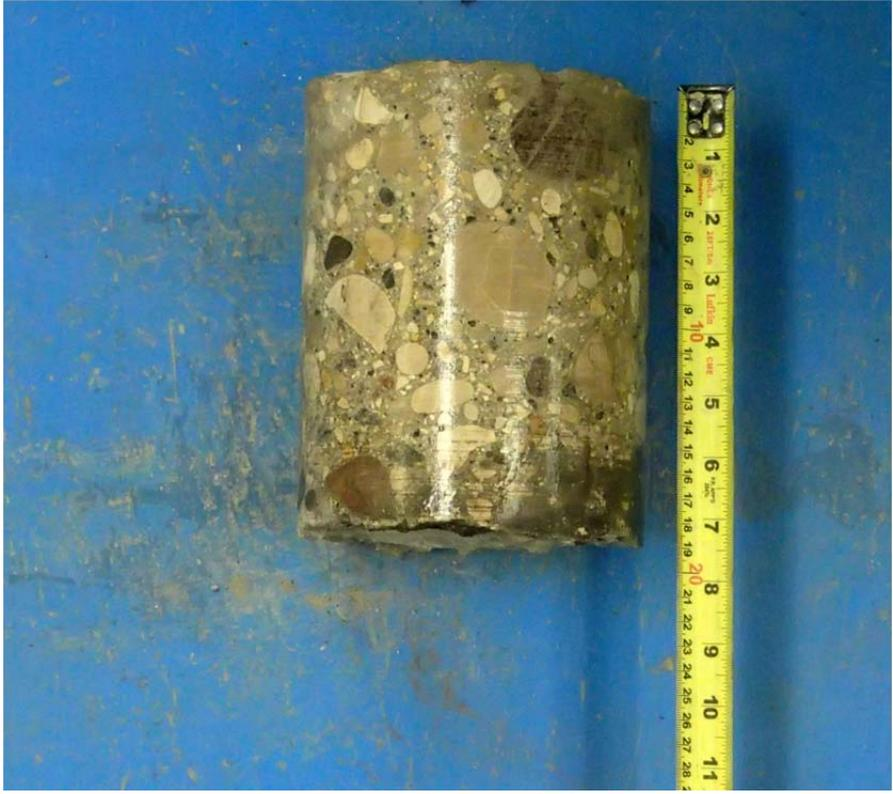
Core sample from Testhole TH4
