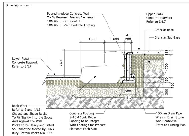
4 ROCK WORK AND RETAINING WALL SECTION
