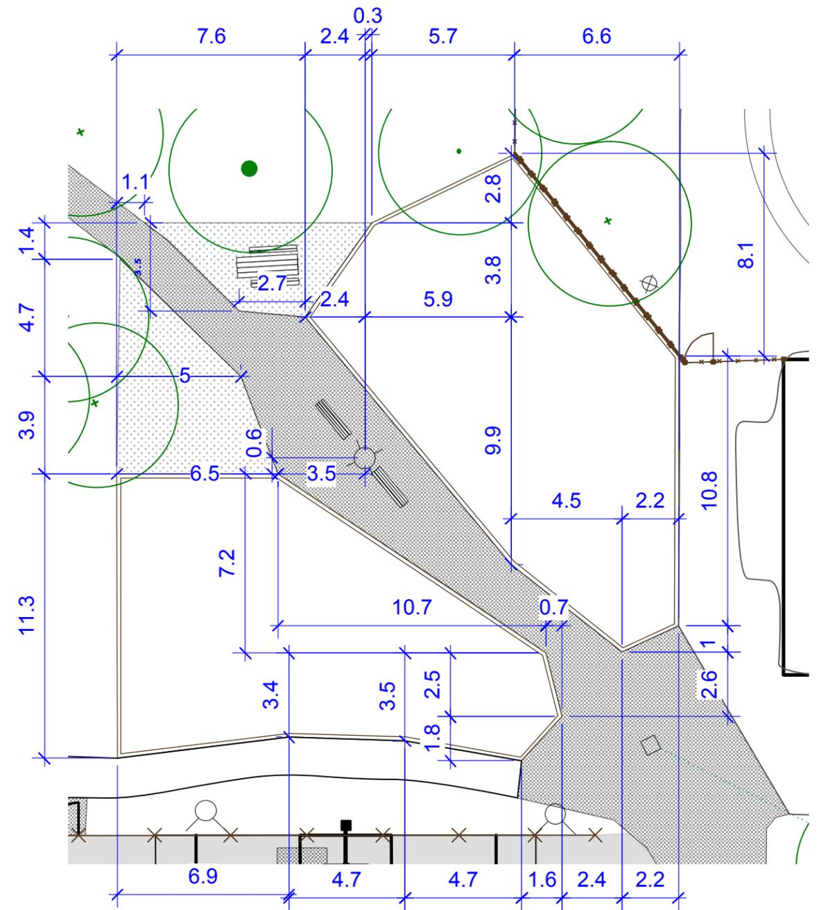
• All dimensions are in meters and are to the outside edge of the timber edging. Contractor must ensure appropriate safety zones for existing and proposed play equipment (based on the latest CSA playground standards) are met. The required safety zones will over-rule any dimensions shown on these drawings. If there is a conflict the Contractor must discuss on site with Contract Administrator. All layouts must be approved by Contract Administrator prior to building.
