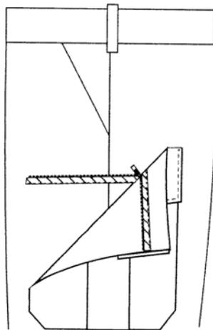
Top of the zipper tape is stitched to the back side of the under pocket patch. The lower edge of the zipper is set to the side pant before closing the patch pocket. The pocket zipper finishes about 1" from the top edge of the flap.
