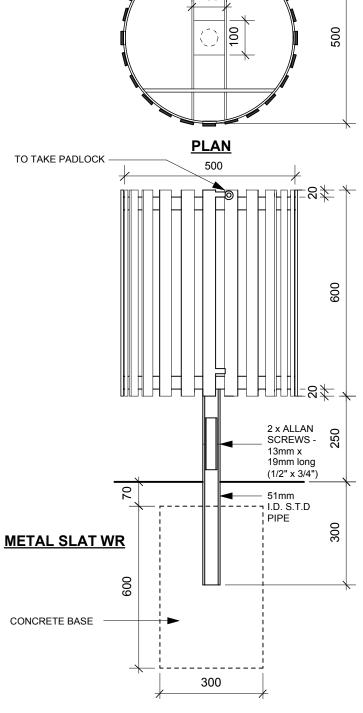
DIMENSIONS SHOWN ARE IN MILLIMETRES UNLESS OTHERWISE SPECIFIED
